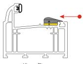
Fit a Frame Wedge "A" to include the packer "B" on the outer frame in the stay fixing area as shown
